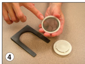
4 Ensure the stainless steel support screen is in place in the bottom of the filter cassette.
