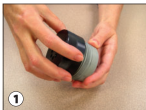
Unscrew impactor inlet from exhaust.
