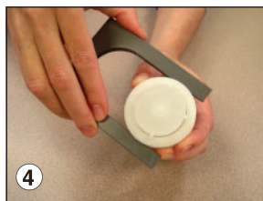
Locate recessed area on filter cassette top and remove impaction disc. If chemical analysis of larger particles is desired, place in appropriate container for shipping to a laboratory for analysis (see Ordering Information, Accessories for glass jars ).
