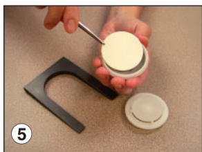
Use forceps to remove collection filter and place in appropriate container for shipping to a laboratory.
