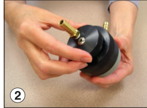
2 Screw calibration adapter onto impactor inlet.
