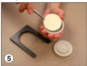
5 Using forceps, place a preweighed 47-mm filter on the support screen.
