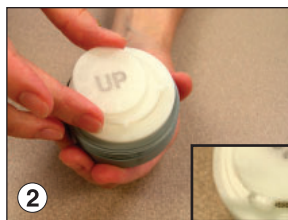
Locate recessed area on filter cassette top and remove impaction disc. If chemical analysis of larger particles is desired, place in appropriate container for shipping to a laboratory for analysis (see Ordering Information, Accessories for glass jars ).
