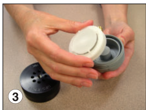
Gently lift filter cassette from exhaust.
