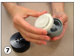
7 Reinsert cassette into impactor.
